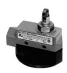
Enclosed Switches Series E6: Cross Roller Plunger (90°; Rotated Plunger) Actuator; 1NC 1NO SPDT Snap Action; 0.5 in - 14NPT conduit
